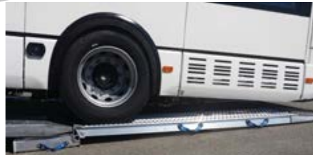
Aluminum bus loading ramps
