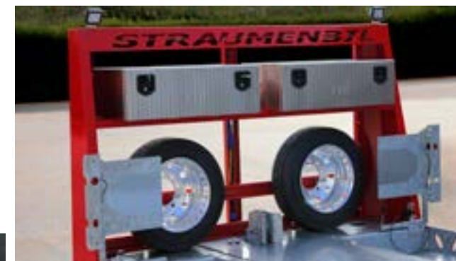
Front sidewall, inox toolboxes, spare wheels
